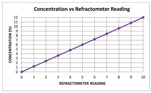
Typical starting dilution for HYDROSOL 5035HB is 5% for most applications and the range is between 4% and 12% depending upon metal being machined and type of machining operation. For concentration control use refractometer; calibrate refractometer with water often, must read 0.0. Always add coolant to water. Typical use concentrations:
